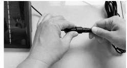
Press the switch once to activate the lights. You will see the pair of lights flash when pressed.
