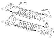
Install screw and screw cap 2 on upper tier and down tier o, then fix to the frame A, Then put cup holder o, cutlery holder f, drip tray or cutting board holder on the tier, finally, install end-caps and anti-slip mat or long anti-slip mat or long anti-slip mat or
